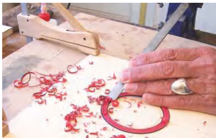
STEP 6. Levelling the rosette with a paring chisel
